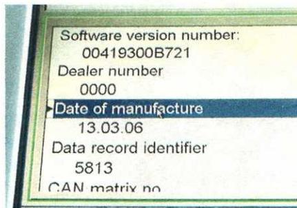
The computer interrogation is vital to understanding the internal health of the potential purchase. Porsche's factory diagnostic computer stores such important data as number of miles versus number of hours driven, helping determine how the car was driven, and any crash events.
