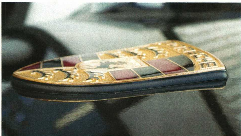
The Porsche hood crest—and the hood itself—can be damaged when pressure is applied to the emblem to close the hood.
